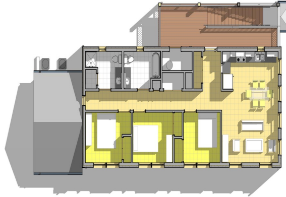
Above: Sample Floor Plan of 3 Bedroom, 1 3/4 Bath Unit. Picture is for informational purposes only.
